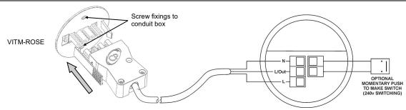
Where absence detection or override is required, wire the switch directly to the detector or use the VITM4 series of marshalling boxes
