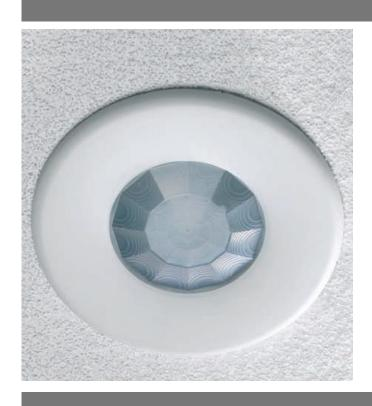
The VITMR-EBDSPIR-PRM PIR (passive infrared) presence detector provides automatic control of lighting loads. This sensor is supplied pre-wired with a 3m lead and include a ceiling rose for ease of installation.
